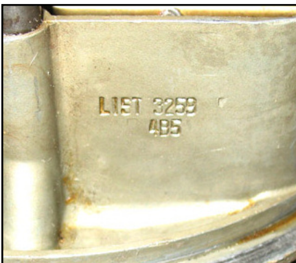
The original carburetors had the List number and a three character date code. That's all. Seems kind of a shame to pay big bucks for so little.
